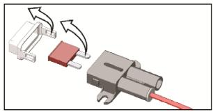
Put the seal on the conductor until it adheres to the fuse holder checking that it has been inserted properly.
