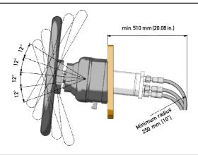
2 Fix bracket (1) supplied with tilt X66 to dashboard (2) following the instructions supplied with tilt X66.
