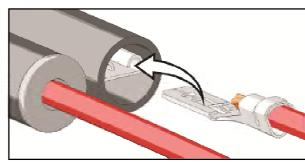
Place the fuse in the fuse holder and put the proper transparent cover.
