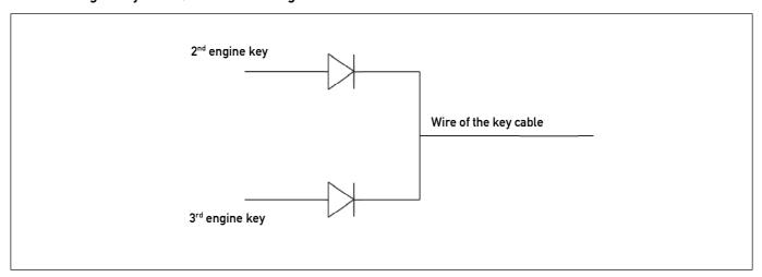
The installer must use diodes with the following minimum features:
