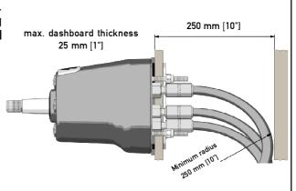
2 By using the proper template supplied with this manual, make the holes (1) for installation in the suitable position on the dashboard.
