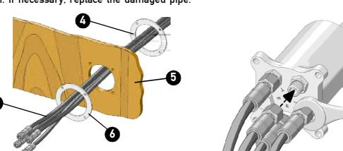
Connect the hydraulic holes UFLEX kit OB-MD as shown in the picture on page 19 for single station applications and on page 21 for dual station applications.
