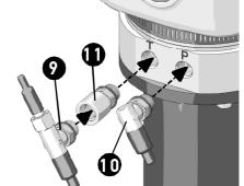
Remove the protection plugs from the fittings, then connect the proper hydraulic hoses as shown in the "Hydraulic connection layout" on page 19 for single station applications and on page 21 for dual station applications.
