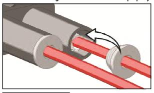
Insert the faston into the free space of the fuse holder.
