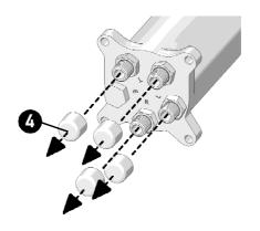
6 Connect the hydraulic holes UFLEX kit OB-MD between the helm and the power unit and the hydraulic hoses UFLEX kit OB-SVS between the helm and the cylinder as shown in the picture on page 19 for single station applications and on page 21 for dual station applications.
