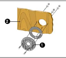
3 Fix the helm to bracket (1) supplied with tilt X66 by using the three M6 screws (3) supplied with tilt X66 following the instructions provided with tilt X66.
