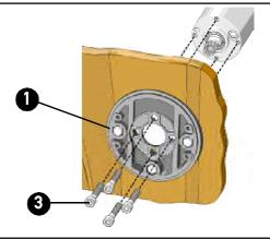
4 Position mechanism X66 putting it on the helm shaft.
