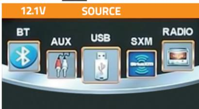
1. Turn the MFD clockwise or counterclockwise to alternate between the available sources; SXM, RADIO, BLUETOOTH, AUX, & USB.
